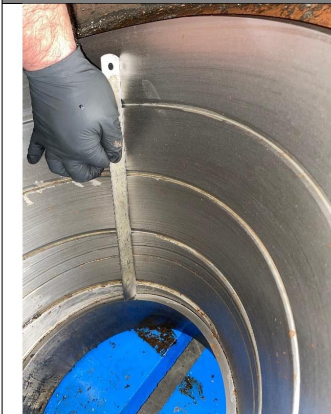
FIG 7 – Shallow Grooves in Liner
