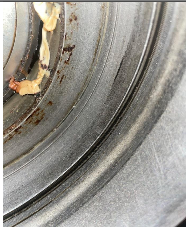
FIG 7 – Shallow Grooves in Liner
