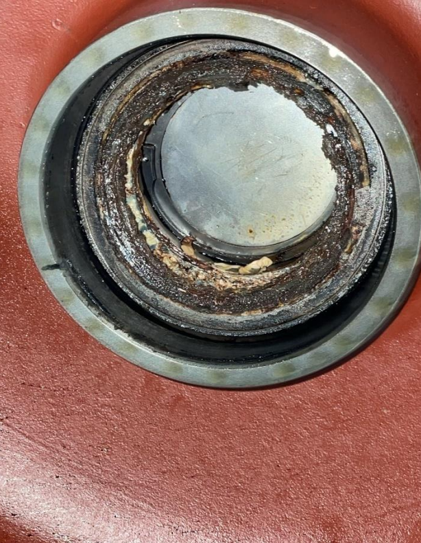
FIG 3 – Upper Bearing Housing as Received
