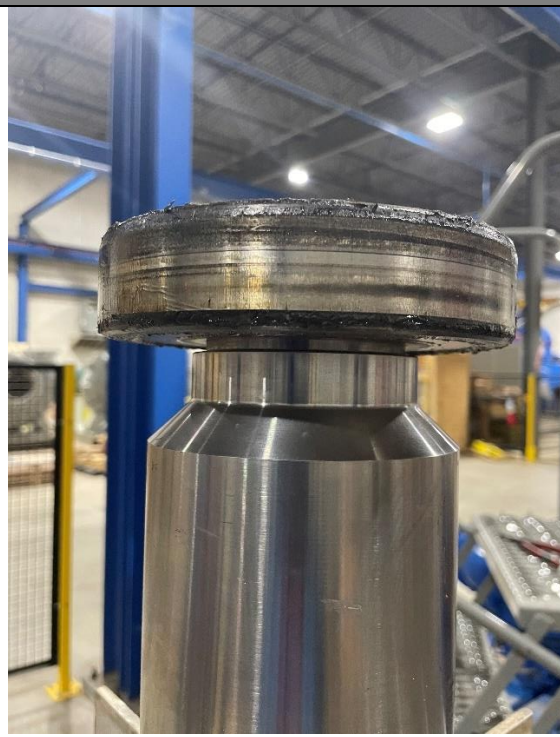
FIG 8 – Worn Outside Edge of Impeller
