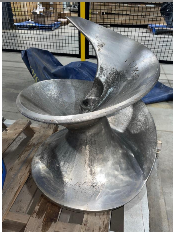
FIG 8 – Worn Outside Edge of Impeller
