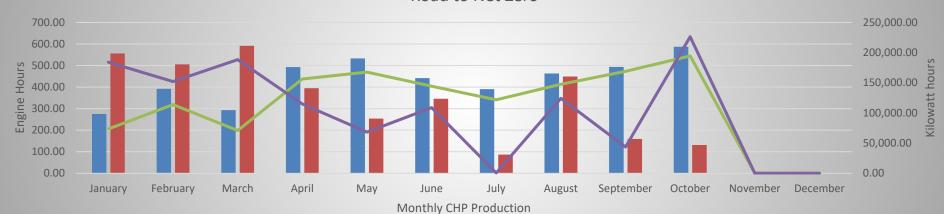
Engine #1 Hrs Engine #2 Hrs ——Engine #1 kWh ——Engine #2 kWh
