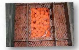
Figure 4-3: WWETCO: Flex Filter
