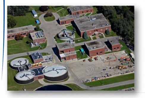
to 58.0 MGD from the Village of Lombard's combined sanitary and storm sewer system. Flow exceeding 58.0 MGD is diverted to two lagoons, which have a design capacity of 14.5 MGD. Both facilities provide wastewater treatment and ultimately discharge to the East Branch of the DuPage River.
